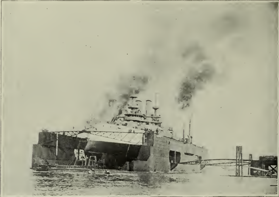
DOCKING THE BATTLESHIP "ILLINOIS" IN THE FLOATING DRY-DOCK AT THE U. S. NAVAL STATION, NEW ORLEANS, LA., JANUARY, 1902.
